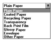
The Print Media <u>Combobox</u> is used to define the type of print media (such as plain paper, or Transparency film) that is loaded in the Canon Bubble Jet printer. This setting is important for controlling the quality of the final printed image. Specifying the correct Print Media setting is essential for producing high-quality printed images.
